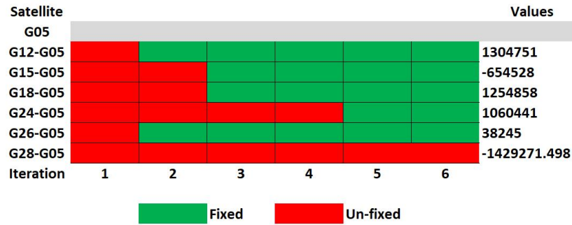
Figure 1: The subset ambiguities fixing (on the first GPS frequency) for a representative epoch, 00:30:00 on 17 July 2014 (DOY 198). The horizontal axis represents the consecutive EKF iterations, the vertical axis indicates the pair of GPS satellites for forming the double-differenced ambiguities.
