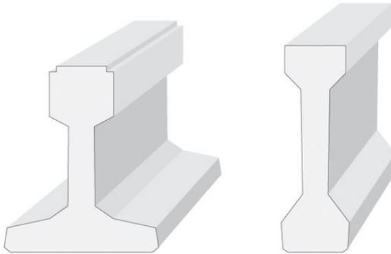
**Figure 3-5 - Example of an M-beam<sup>6</sup> (I-beam with wide bottom flange) and an I-beam (source: [http://www.scib.com.my/prestressed\\_beam.html](http://www.scib.com.my/prestressed_beam.html))**
