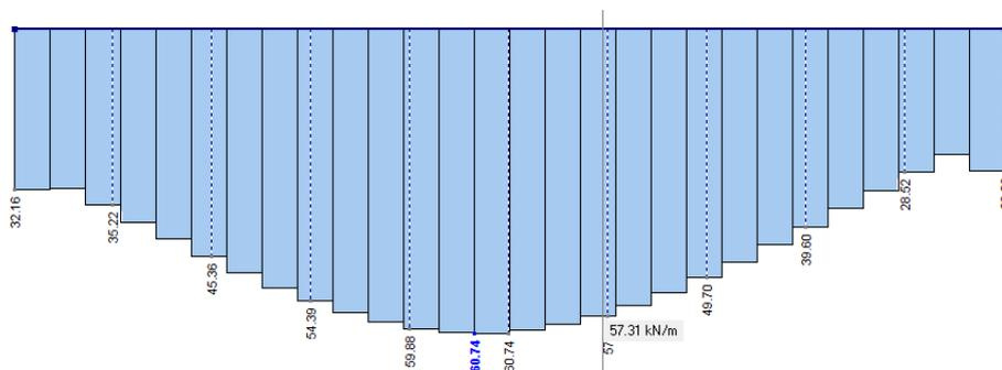
Appendix Figure 6-4 Shear force due to LM1 axles. (span: 19m, bedge = 4m,  $E_y = 11 \text{ GPa}$ ,  $h = 950 \text{ mm}$ )
