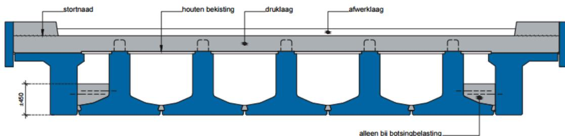
**Figure 3-4 - cross-section ZIP bridge [14]**
