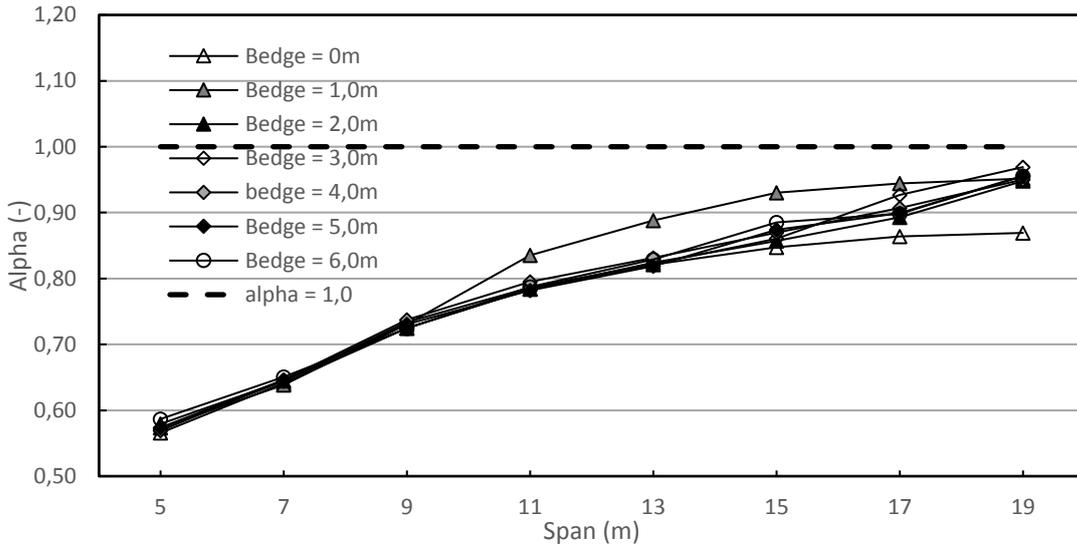
**Appendix Figure 9-11 - A factor (Shear force) for the comparison of Load Model 1 and the Asphalt Lorry for different spans and edge widths**
