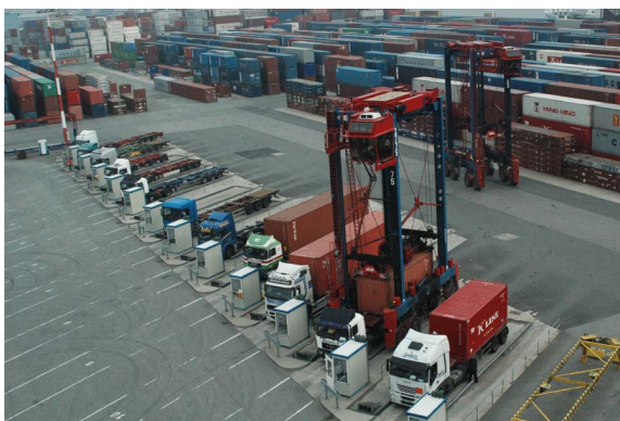
(a) Straddle carrier (un)loading trucks with containers [author = unknown, retrieved 16/07/2018]
