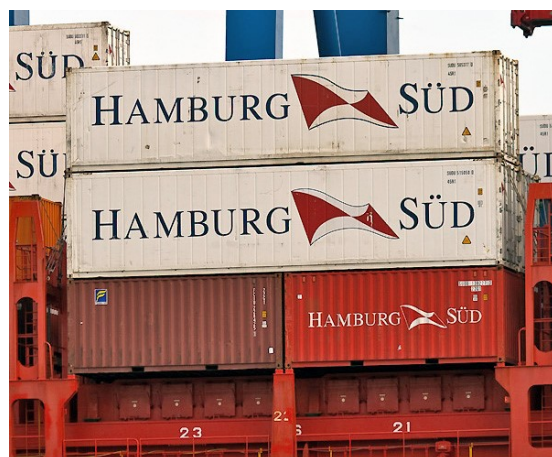
(a) Example of a FEU containers stacked on top of two TEU containers [Bätge, 2009]
