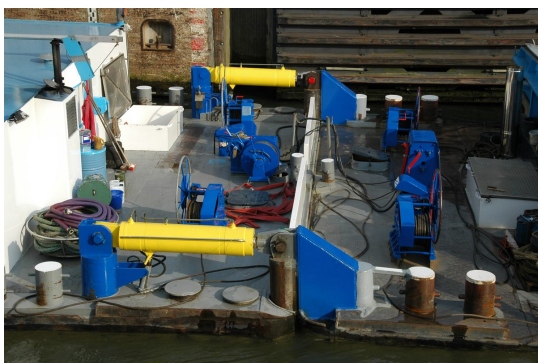
(a) Hydrologic barge coupling system. [Van Huizen, 2014]
