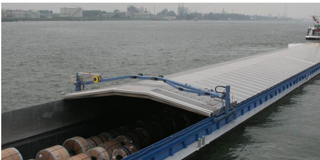
Figure 8.2: Example of an existing hatch cover crane [Blommaert, retrieved 12/10/2018]
