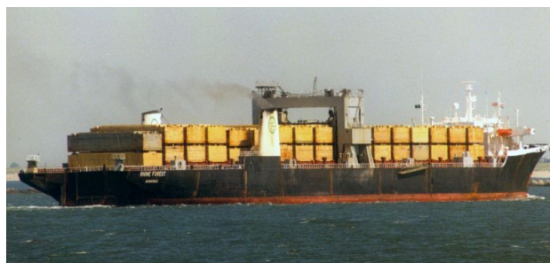
(b) MV Rhine Forest, LASH-carrier, loaded with yellow collared lighters. This vessel is equipped with a gantry crane enabling the (un)loading of lighters aft of the stern. [Seyler, 1998]
