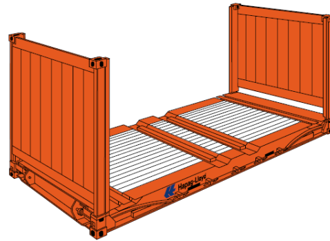
(b) Example of a Flatrack container [Hapag-Lloyd AG, 2016]
