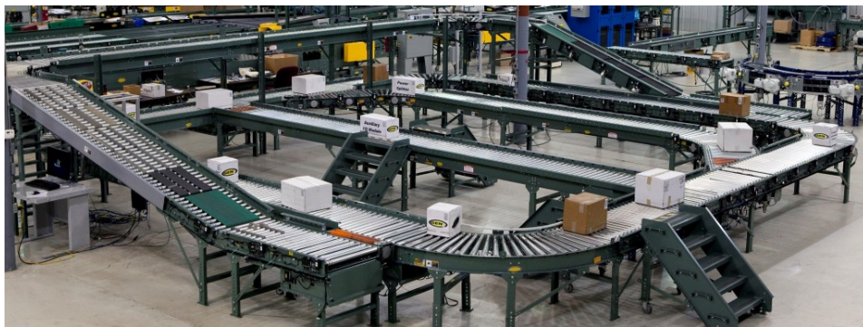
Figure 8.7: Example of a multilevel rolling conveyor system [Conveyor Handling Company, retrieved 16/07/2018]
