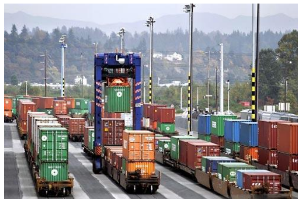
(b) (un)loading carriages with stacked containers in the Port of Tacoma, USA. [Ringman, 2005]
