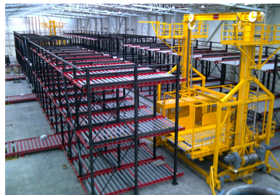
(b) Baku Cargo Terminal 20ft Elevating Transfer Vehicle [BDP, retrieved 13/07/2018]
