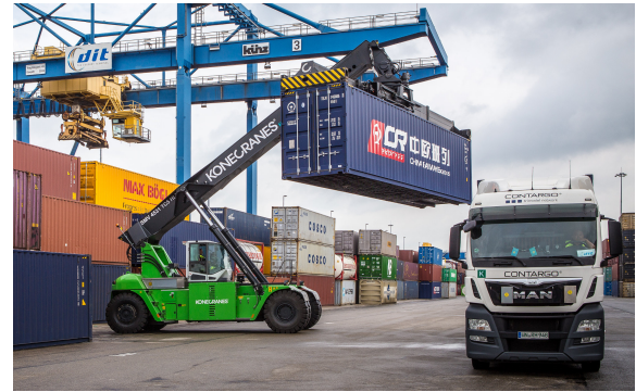
(b) Truck (un)loading with reach stacker. [Management, retrieved 12/04/2018]
