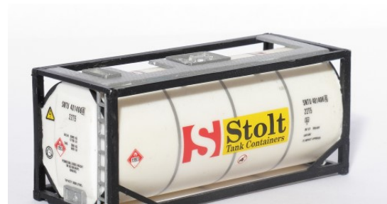
(d) Example of a Tank container [C Rail Intermodal, retrieved 28/02/2018]
