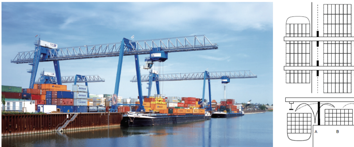
Figure 5.5: Wide-span gantry crane: real world application and schematic operations overview. [Rademaker, 2007]
