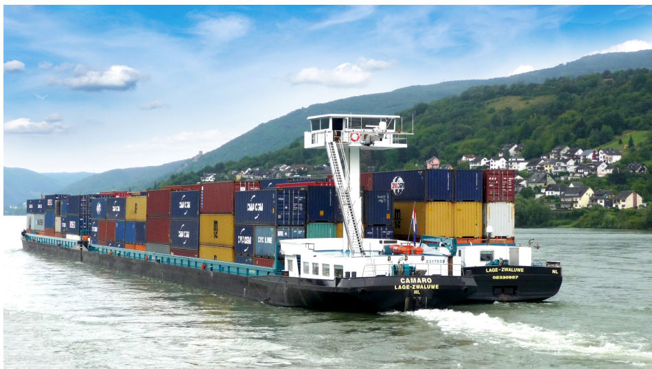
Figure 3.5: MV Camaro (CEMT Va) pushing a container barge (CEMT E II) while also having two barges alongside it (CEMT E II in a long version and an E II in short edition.) [found on MarineTraffic.com, year = unknown]
