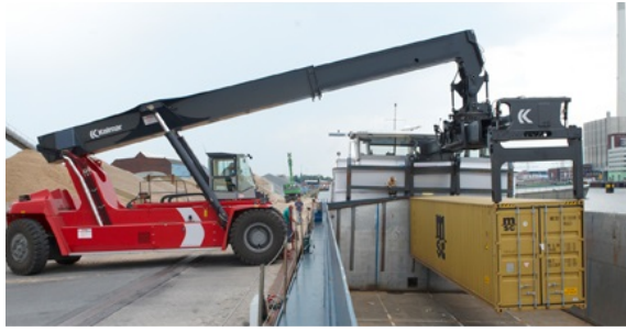
(a) Vessel (un)loading with reach stacker. [Translink, retrieved 12/04/2018]
