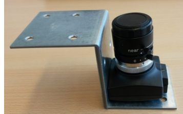
Figure 6.12: Structure holding the optical camera
