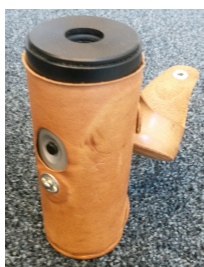
Figure 3.6: Pistonphone of Brüel and Kjaer Type 423
