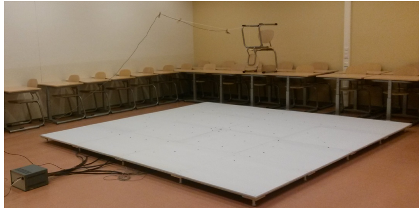
Figure A.2: Set-up for the verification of the complete acoustic camera
