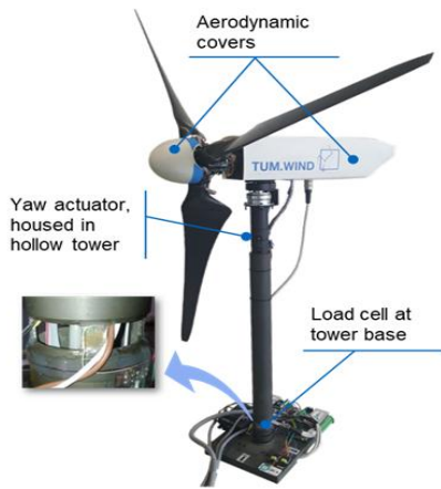
Figure 3. The G1 wind turbine with highlighted components.
