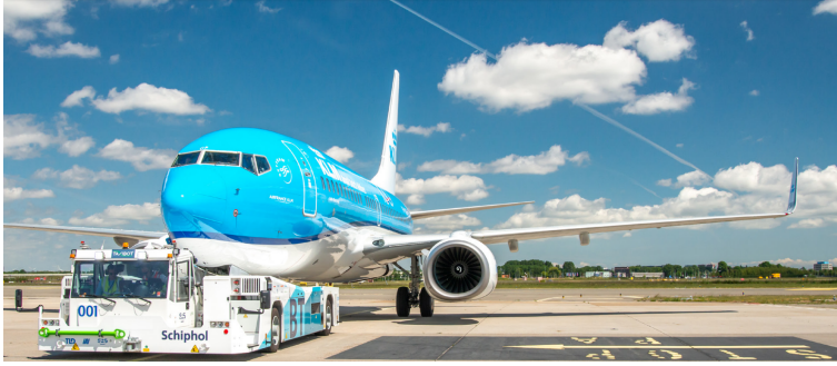
Figure 1.1: External electric towing vehicle towing an aircraft at Amsterdam Airport Schiphol [144].
