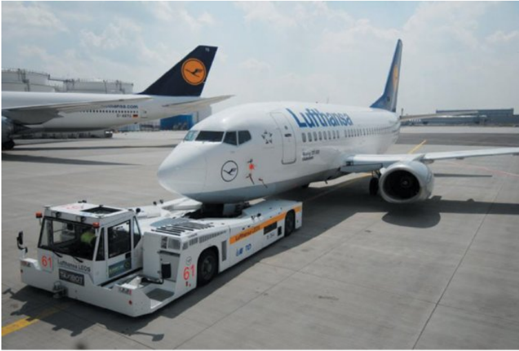
Figure 2.2: TaxiBot in operation at Frankfurt Airport [157].
