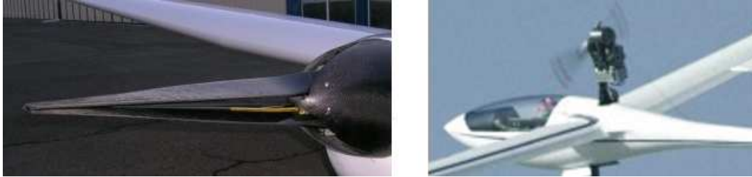
Figure 4.19: a: Foldable propeller in folded position b: Retractable propeller, in operation on PIK-20 aircraft
