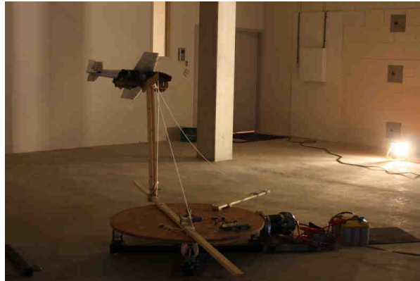
Figure 4.34: Test set-up of rotating platform with aircraft attached
