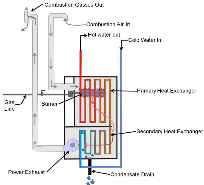
Figure 2.1: Schematic overview of a condensing boiler<sup>2</sup>
