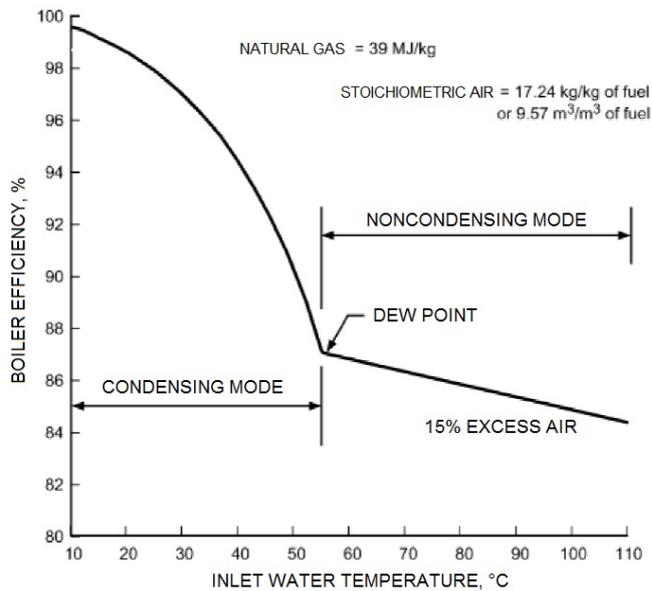
Figure 2.2: Efficiency curve of a condensing boiler. Note how the efficiency rises sharply above the dew point of the exhaust gasses<sup>3</sup>
