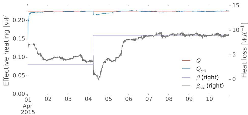
Figure 5.7: Tracking  $Q$  and  $\beta$  when  $\beta$  suddenly increases significantly, without tuning the covariance matrices
