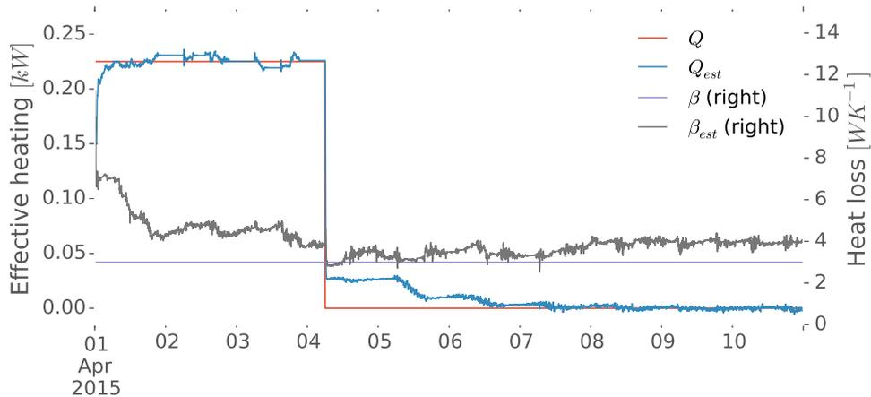
Figure 5.5: Tracking  $Q$  and  $\beta$  when  $Q$  suddenly drops to zero.
