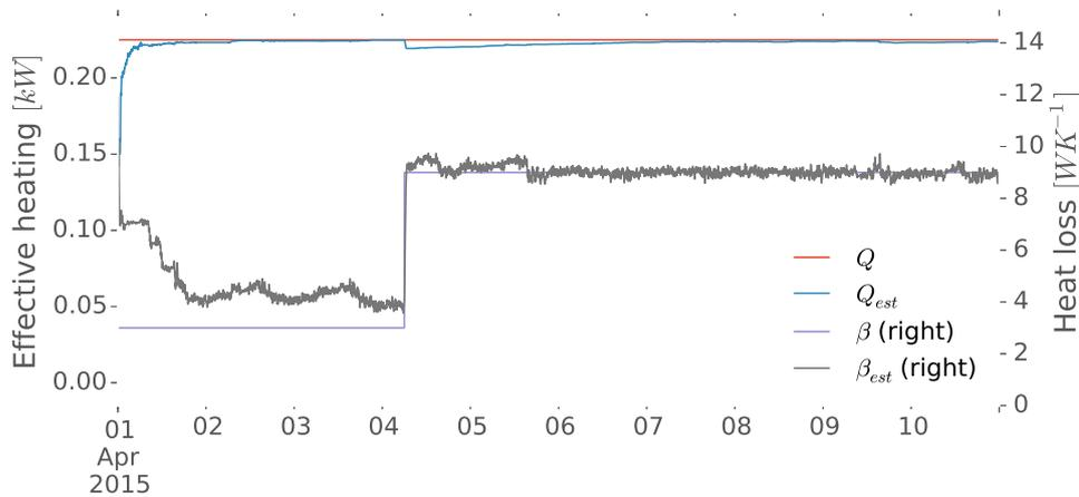
Figure 5.9: Tracking  $Q$  and  $\beta$  when  $\beta$  suddenly increases significantly, with tuned covariance matrices for this specific failure
