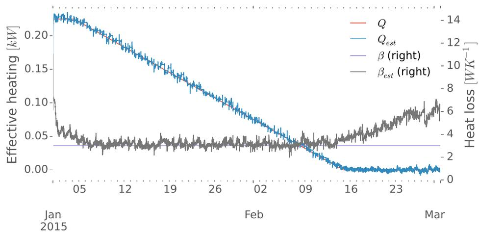
Figure 5.11: Tracking  $Q$  and  $\beta$  when  $Q$  slowly drops to zero.
