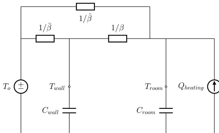
Figure 3.3: RC Diagram of heated house model
