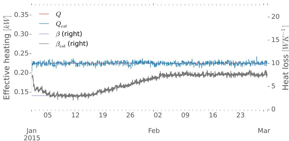
Figure 5.12: Tracking  $Q$  and  $\beta$  when  $\beta$  slowly increases.
