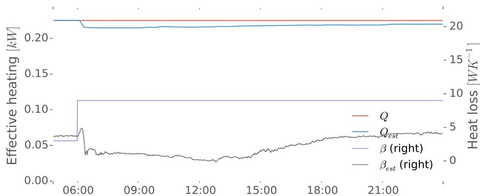
Figure 5.8: Detail view of the sudden increase in  $\beta$ , without tuning the covariance matrices
