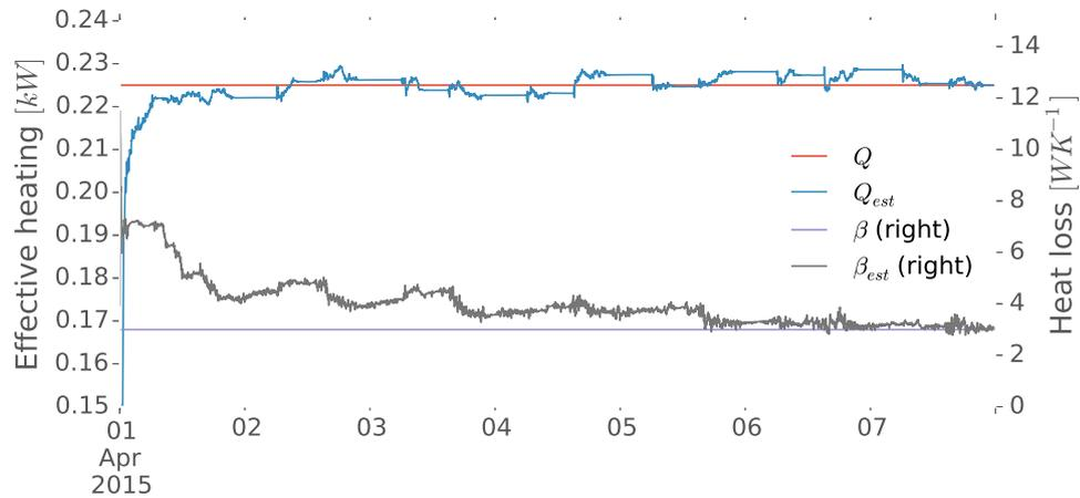
Figure 5.4: Tracking  $Q$  and  $\beta$  in the presence of additive measurement noise
