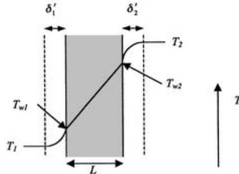
Figure 3.1: Conduction and convection around a wall.<sup>1</sup>
