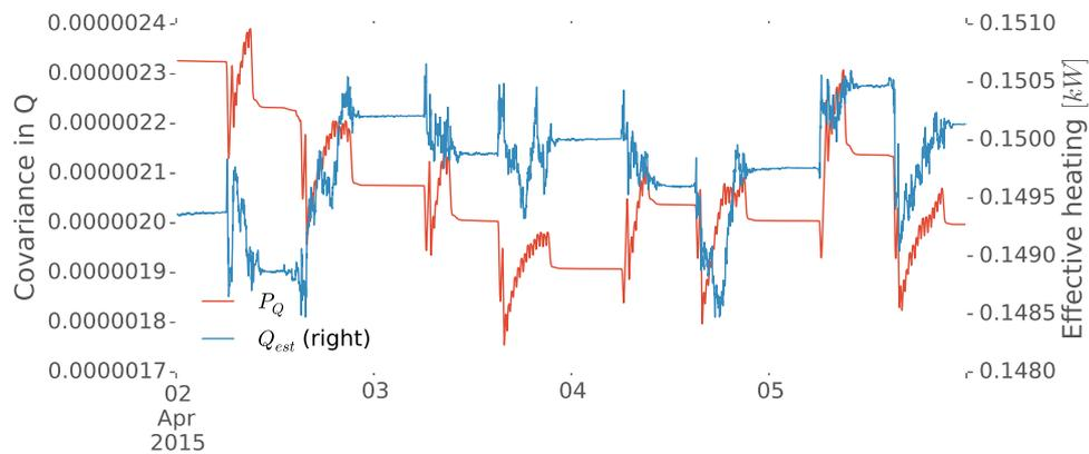
Figure 5.17: Effect of ad-hoc approach limiting the windup of covariance, resulting in more stable tracking of  $Q$
