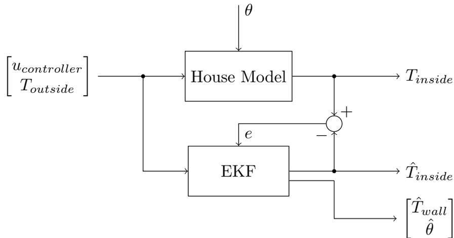
Figure 5.1: Schematic overview of parameter estimation setup using the Extended Kalman Filter (EKF).
