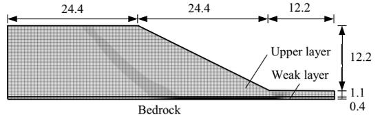
**Figure 1.** Finite-element mesh of the slope example and its deterministic critical slip surface (Unit: m)
