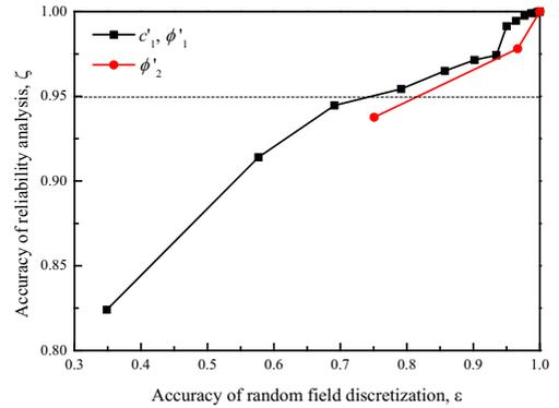
**Figure 5.** Effect of accuracy of random field discretization on accuracy of reliability analysis
