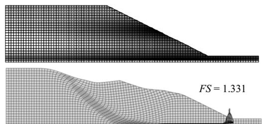
**Figure 2.** A typical realization of cohesion random fields and its slope stability analysis results
