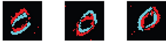
Figure 3: Saccades on the N-MNIST dataset, red=on (pixel changes from black to white), blue=off (pixel changes from white to black), from [8].
