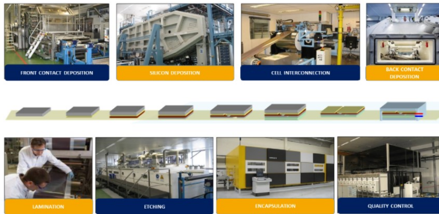
Figure 1.7: Production process for a-Si modules at HyET Solar [27]
