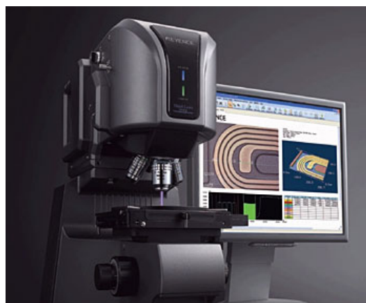
Figure 3.7: Schematic representation of Keyence confocal Microscopy Setup used at TU Delft [64]
