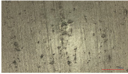
(a) 3D confocal microscope image for untreated Al Roll
