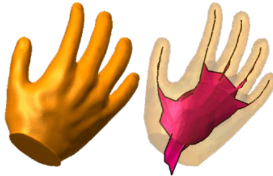
Figure 2.2: 3D MAT of a surface model of a hand [Amenta and Kolluri, 2001]
