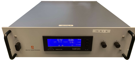
Figure A.6: SM 500-CP-90 bidirectional power supply from Delta Elektronika
