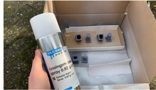
Step 2: Apply release agent to molds
