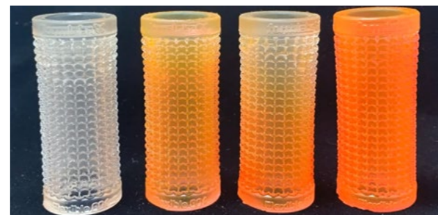
Figure 11.4: Coloring flexible 80A. Soaking in IPA and alcohol ink.
