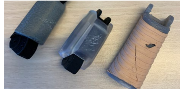
Figure 11.3: Grip material scratch test. Cuts made with simple kitchen knife.
