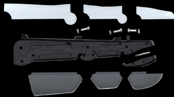
Figure 10.2: Finger exploded view
