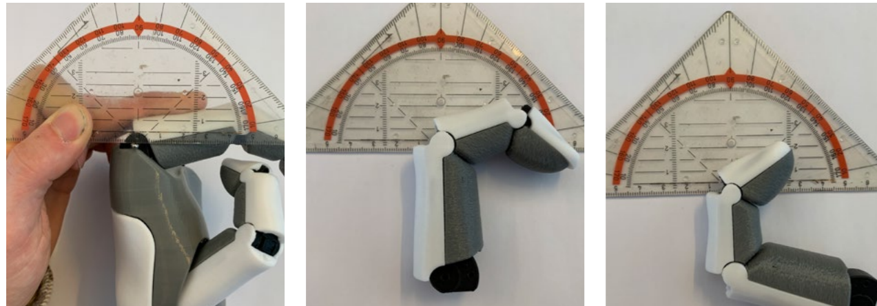
Figure 13.2: Finger flexion capabilities test
