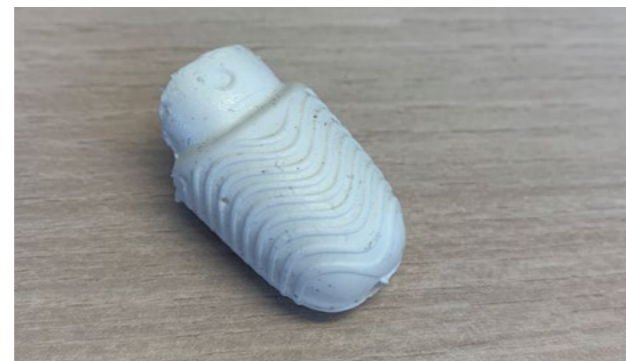
Step 8: Take silicone part out of mold
