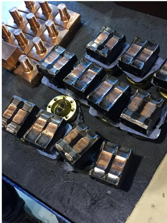
Figure 3.2: Contact wear: grooves by the rolling contacts.
