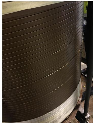
Figure 3.1: Slightly deformed windings
