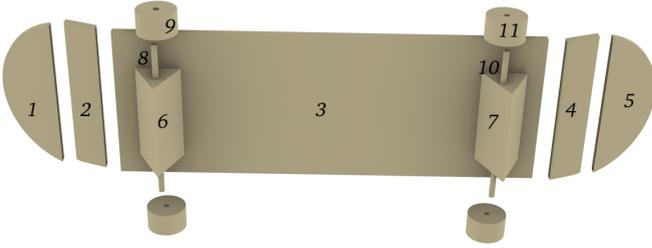
Fig. 7: Clarification on the 11 segment model. Now you can see that there are 13 shapes, but the wheels are taken as one wider cylinder in 2D, which results in 11 segments
