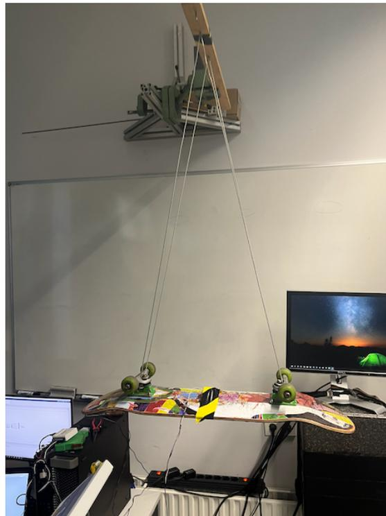
Fig. 27: Test setup for inertia testing
