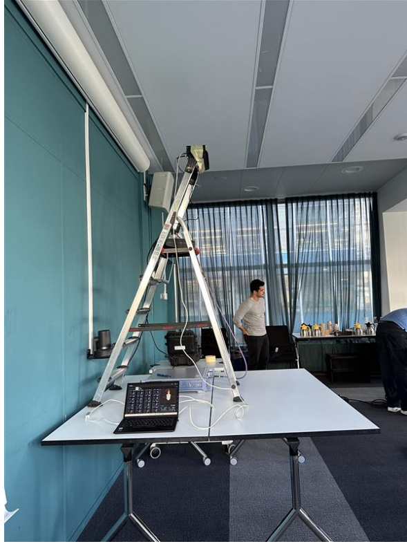
Figure 2.22: The transmitter setup of the measurement
