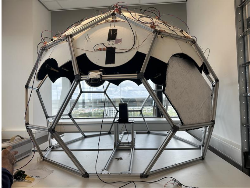
Figure 4.1: Measurement setup of BBox broadside pattern in the Dome
