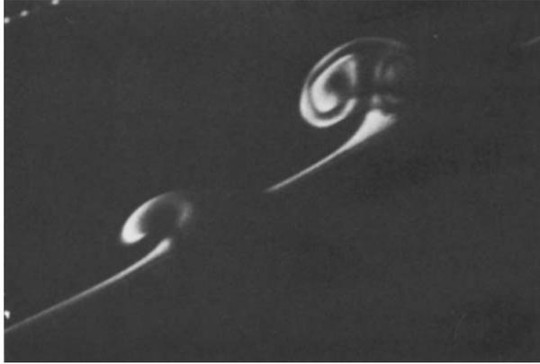
Figure 5.9: Spiral vortex cross-sections on a rotating cone of half-angle  $\psi = 30^\circ$ , taken from Kobayashi et al., 1983.
