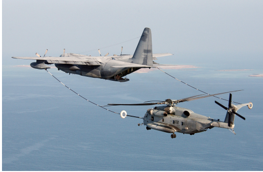
Figure 2.25: A CH-53 helicopter performing an aerial refueling task. (Source: www.defenseimagery.mil)
