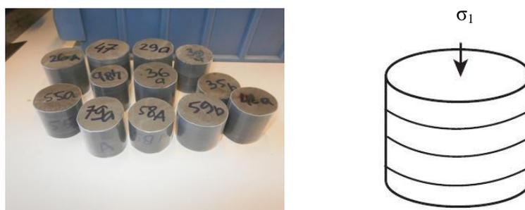
**Figure 1** (a) Photograph of the Whitby shale samples. (b) Loading orientation and bedding plane of the shale sample (Modified from Zhubayev *et al.* 2016).
