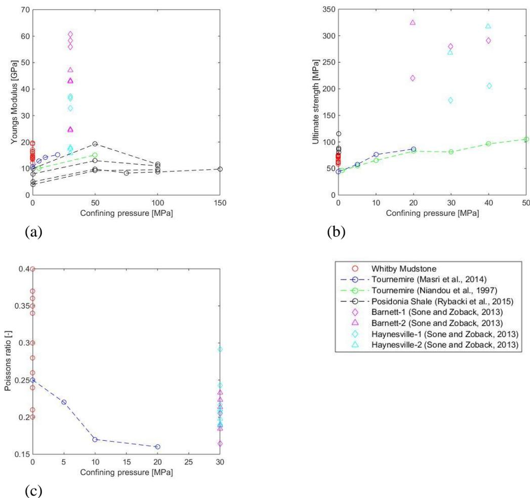
**Figure 3** Relation between confining pressure, Young's Modulus, Ultimate strength and Poisson's ratio from uniaxial and triaxial tests. (a) Confining pressure versus Young's Modulus. (b) Confining pressure versus Ultimate strength. (c) Confining pressure versus Poisson's ratio.
