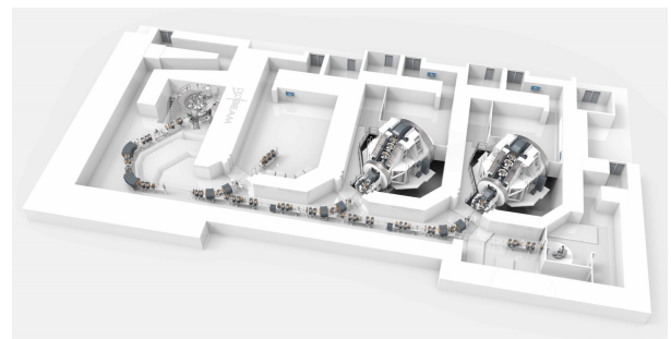
Figure 1: Layout of three gantry treatment rooms for PBT. Protons are guided from the cyclotron to the gantry. This diagram was developed by HollandPTC
