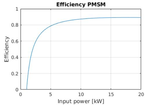
FIGURE 2.3: Efficiency of a 20kW PMSM
