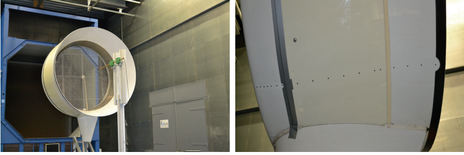
Figure 3.1: Pictures showing the experimental setup with hot-wire anemometer placed on the traversing system (left) and pressure taps located along the duct surface (right).
