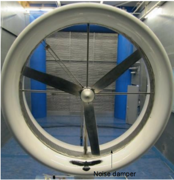
Figure 5.9: Front view of the DonQi ® DWT model used for the experimental study [Ten Hoopen, 2009].
