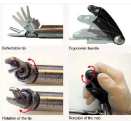
Radius instrument (Tuebingen Scientific, Germany) Mechanism: Gear systems
