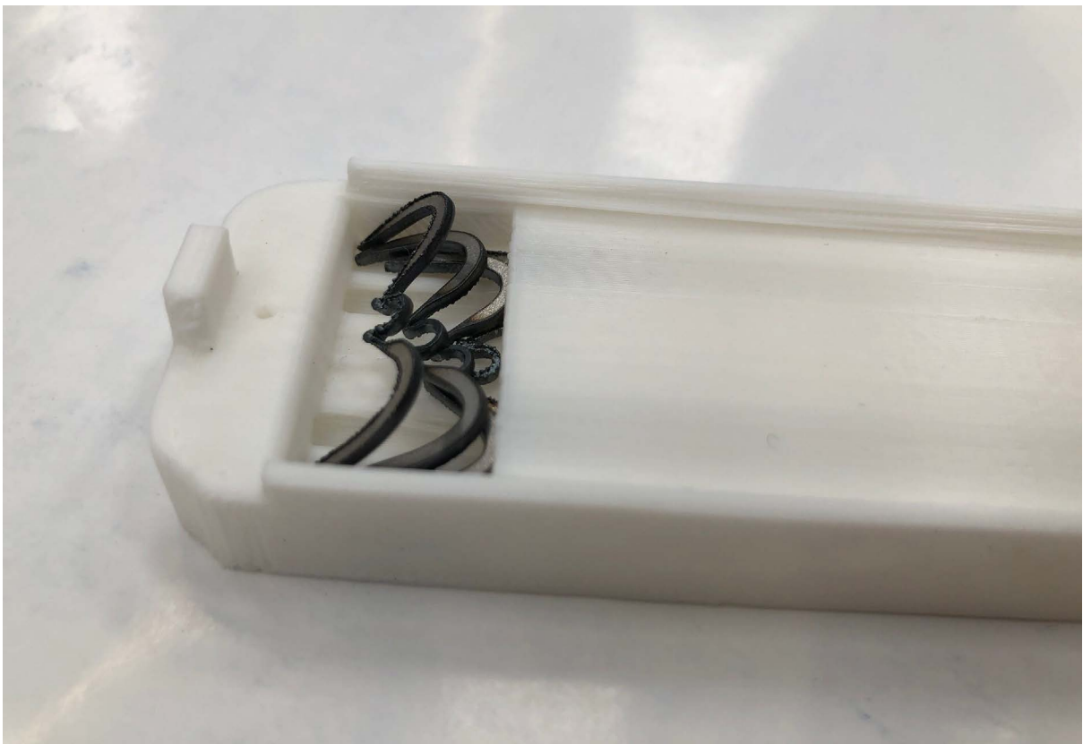
Figure K-11: 90-degree rotation due to staples getting stuck in the bottom corner when using no mechanism at all
