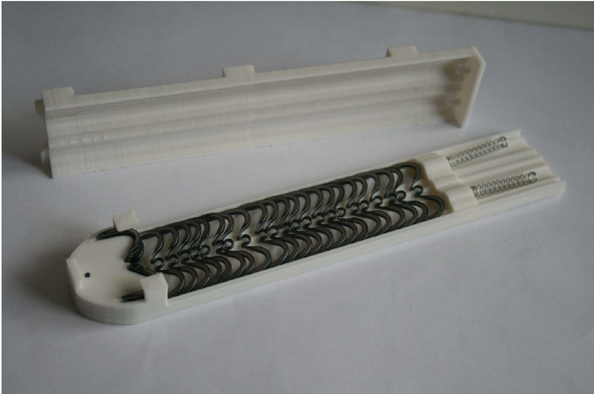
Figure K-16: A bigger 3D printed model of the cartridge, used to test if the mechanism would still work with a bigger amount of staples. Here the springs from pens were used, as I was awaiting new springs to arrive in the mail. These pen springs were not strong enough...
