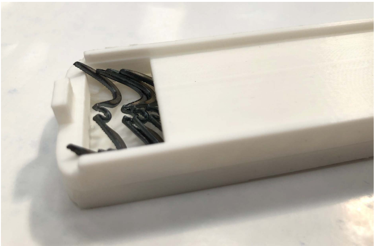
Figure K-9: 90-degree rotation caused by the slide
