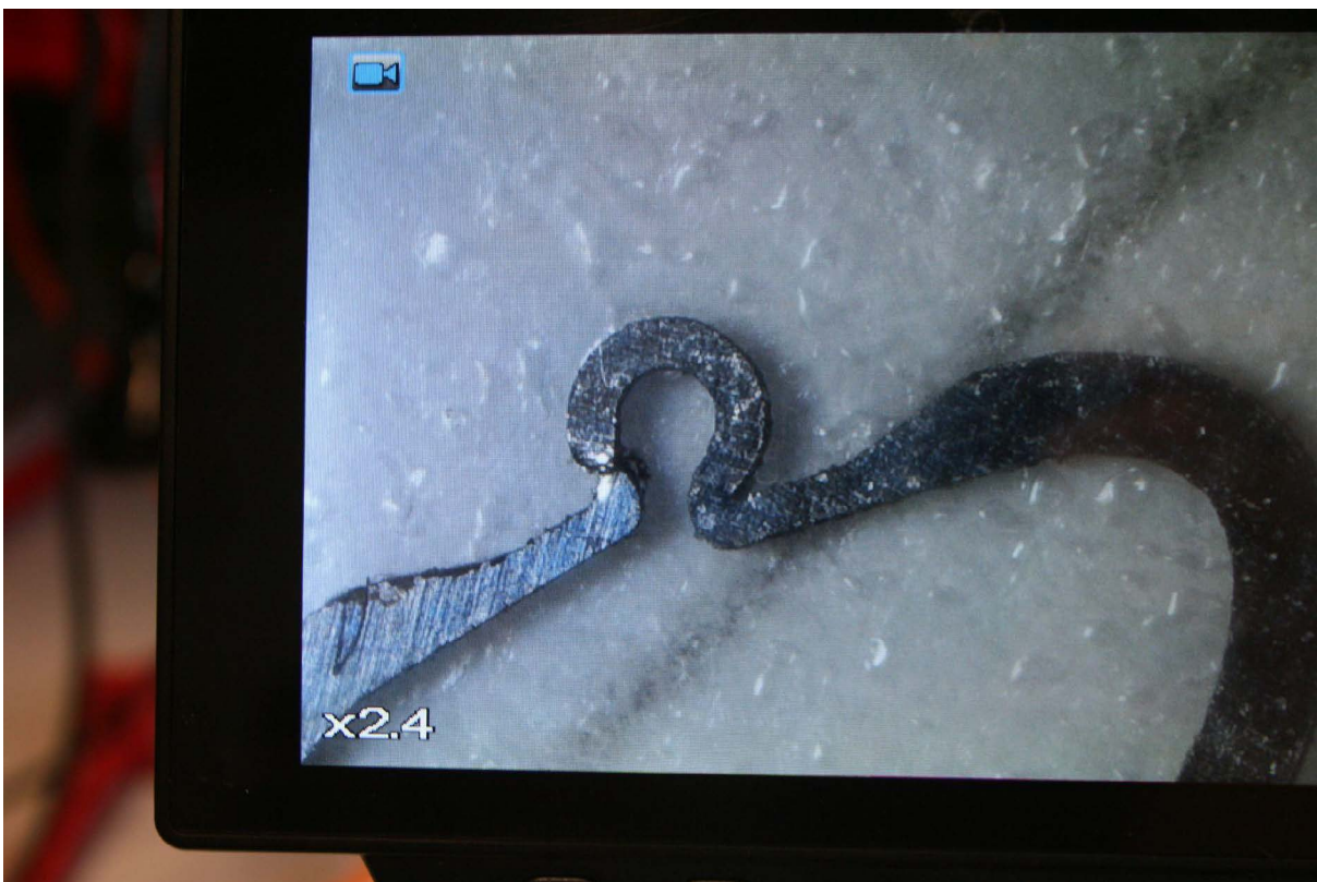
Figure J-17: Another staple with a huge tear at the same location. Zoomed in x2.4.
