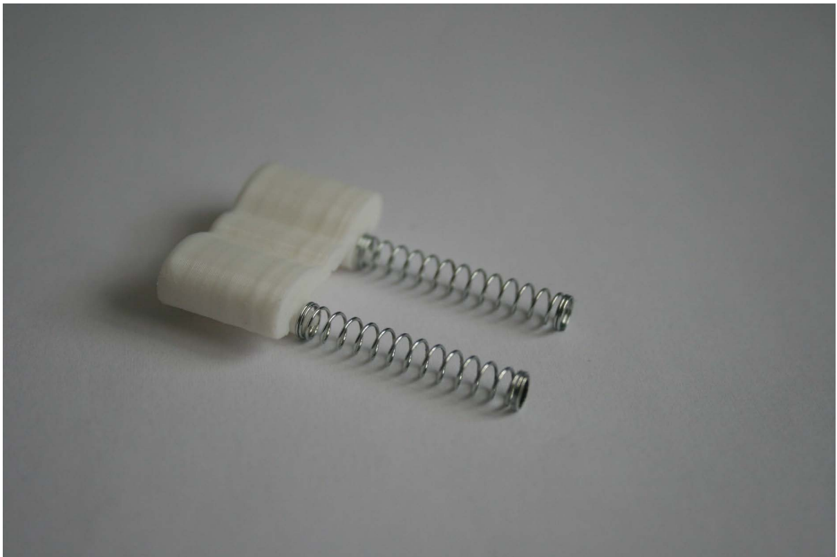
Figure K-14: A 3D printed model of the spring-loaded pushing mechanism.
