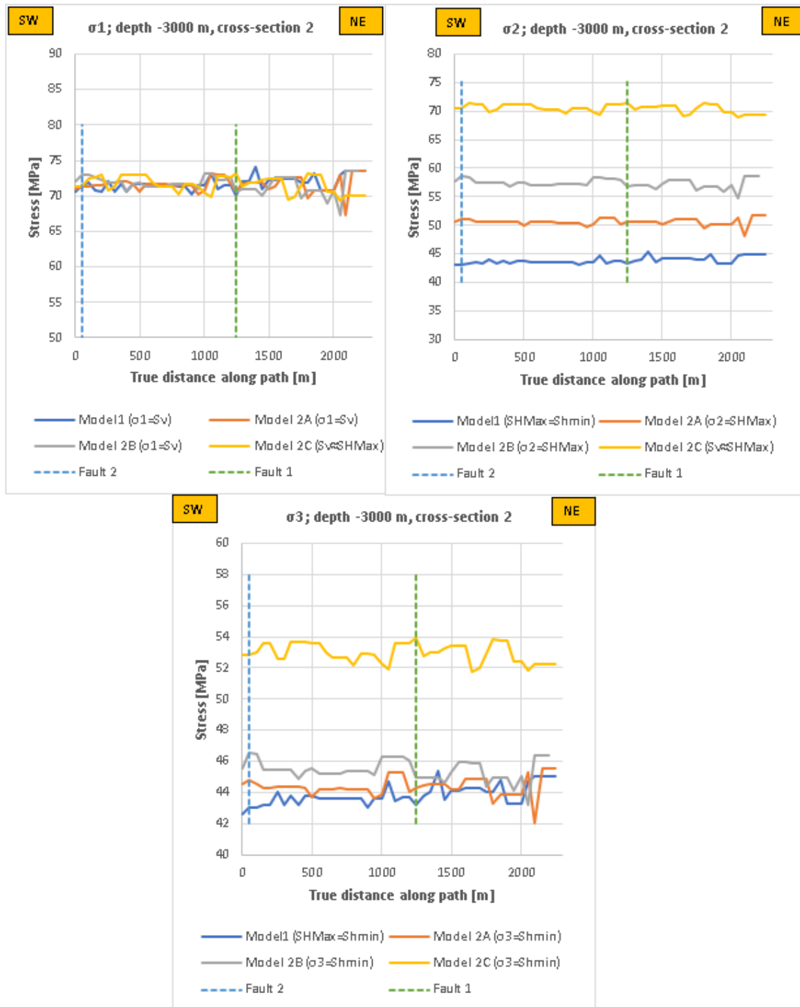
Figure 42. The magnitude of principal stresses in cross-section 2 (depth of -3000 m). Left: Maximum principal stress, right: intermediate principal stress, bottom: minimum principal stress
