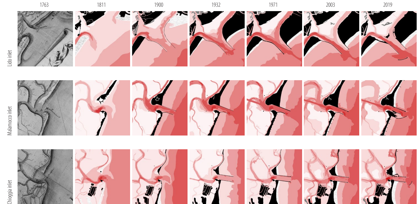
fig. 03/02 Venetian lagoon inlets of Lido, Malamocco, and Chioggia transformation between 1763 and 2019. To be noticed is the progressive deepening of the navigable canals and the construction of concrete sea jetties to funnel water currents. This funnel effect determines the self-deepening of the inlets.
