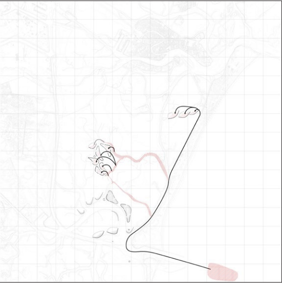
fig. 07/08/08 2023/24 - 3 rd stage: dredges collocation in cluster B While the dredges are pumped within the cluster B, cluster A continue to accumulate additional sediment, growing in elevation.
