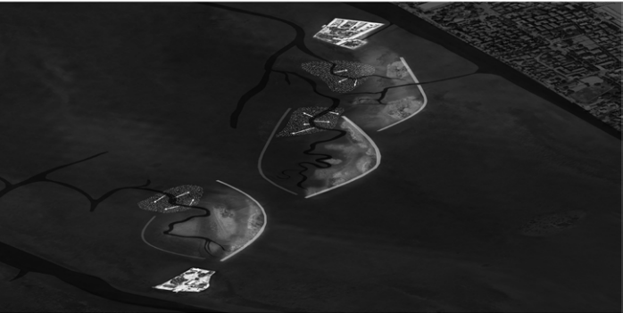
end of 2025 - 4 th stage: underwater vegetation prairies Autoctonous seagrasses of the Venetian Lagoon, Zostera noltii and Zostera marina , are planted where the structures are the furthest from each other. They will naturally contribute, through their spreading and growing, to consolidate those sediments that will be dispersed by tidal alternation.
