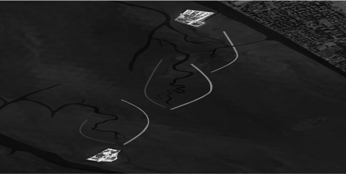
2023 - 1 st stage: excavation and construction Based on the former ones occupying the area at the beginning of XX century and later on erased because of accretion, meandering canals are excavated to promote more efficient tidal expansion: they will be fundamental to promote the natural movement of sediment. The construction of the structures happen in this phase.
