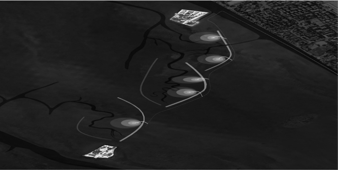
2024 - 2 nd stage: sand nourishment Sand, dredged from just outside Malamocco inlet, is used start the process of natural sedimentation. Through a dredge-boat sand is pumped inside the structures until reaching the desired elevation.
