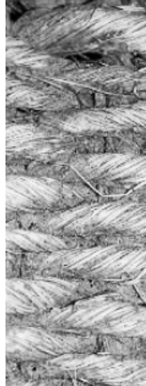
01 fig. 07/08 Examples of biodegradable materials to be used for the structures' production. 01/ Geotextile composed of natural fibres (viscose) derived from cellulose. 02/ Geogrid obtained from vegetable fibres from the agave plant. 03/ Geogrid obtained from wood fibres from the outer shell of the coconut. 04/ Natural fibre geotextile composed of yarns from hemp, Yuta, cellulose and wool.
