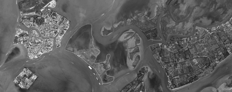
2010 The white dotted line represents the artificial borders of the barene , the built dykes; the white rectangles are the dredgeboats ready to pump sediment inside the created perimeter.
