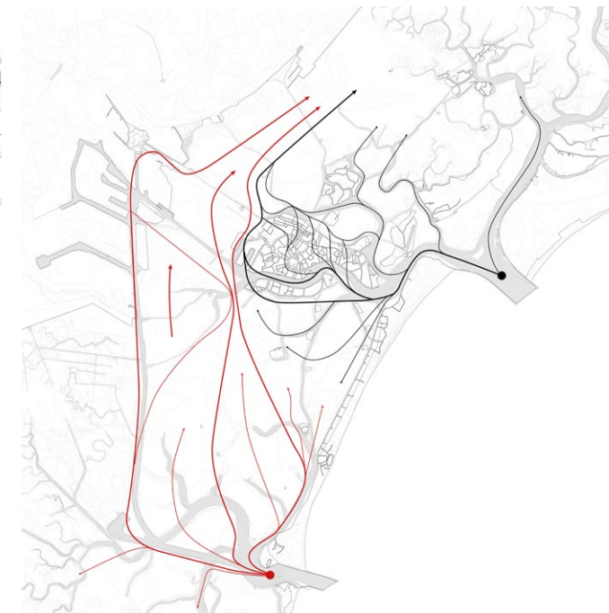
fig. 03/07 Tidal expansion, directions and intensity, from the inlets of Lido (north) and Malamocco (centre) in 2009, after the excavation of Canale Malamocco–Marghera. Visibly, due to the funnel effect characterizing the central inlet of Malamocco, after the excavation of the canal and the construction of concrete jetties in the Adriatic sea, the incoming currents (red arrows) are channelled powerfully in the Canale Malamocco–Marghera. This causes the constraint of the incoming currents from Lido inlet (black arrows) inside Venice's canals. The instability between the red and black arrows have caused the increase of acqua alta events within the last 70 years.
