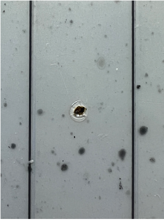
(f) Backside image of a hotspot created during WCSS on R20026-3932
