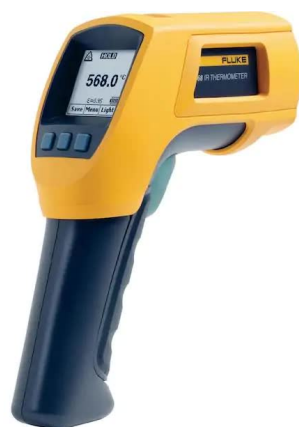
Figure 3.8: Fluke 568 IR Thermometer [22]. This thermometer was used to measure the temperature, but also to validate the temperature map produced in the images from the Fluke Ti32 Camera.
