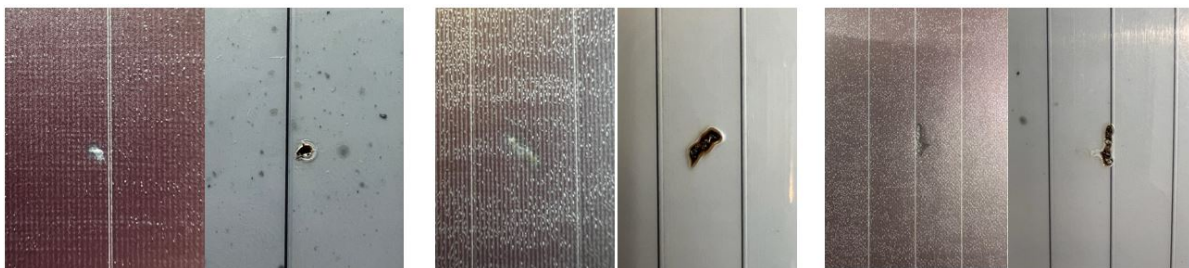
Figure 6.1: Classification of three different hotspots present on the modules. The left image is a 'circular' hotspot, the middle image is a 'linear' hotspot and the right image is a 'linear along the scribe' hotspot.
