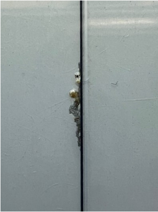
(d) Backside image of a hotspot created during LS at SC on R20026-4096
