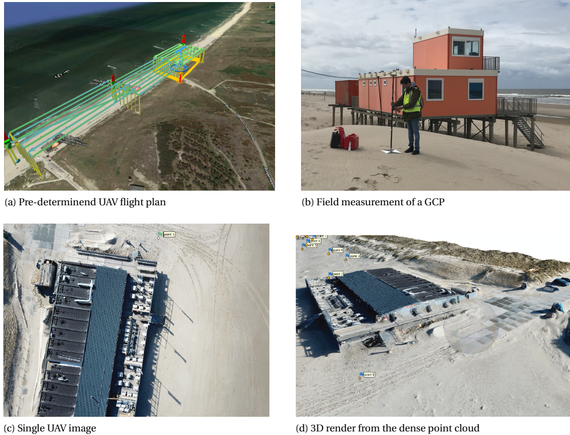
Figure 3.11: Phases in the UAV photogrammetry measuring process
