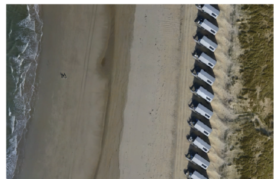
(b) Sediment patterns due to local influence on aeolian sediment transport by ribbon-development
