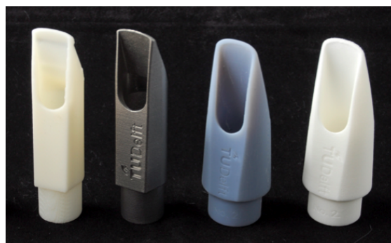
Figure 1: Preliminary mouthpiece models produced using different 3D printing technologies and materials.
