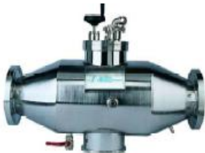
Figure 7-2: Sita UV disinfection module SMP140, with 4 medium-pressure lamps providing >80mJ/cm 2 and a maximum flow rate of 1200m 3 /h (A&C Engineering B.V.)
