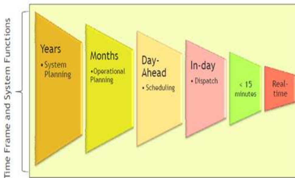
Figure 5.1: Time Frame and System Functions in Regulatory and in Competitive Markets, 1 [1]
