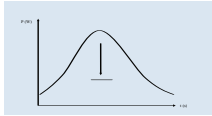
Figure 3.4: Peak Clipping: involves reducing power consumption load during periods of peak demand.
