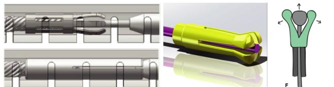
Figure E: Concept F, thicknut mechanism with multiple spikes (left, top), simplified version with only 2 spikes (left, bottom), SolidWorks model (middle)
