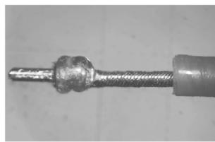
**Fig. 26:** Expanded bellow (left) before pulled into the catheter (right)
