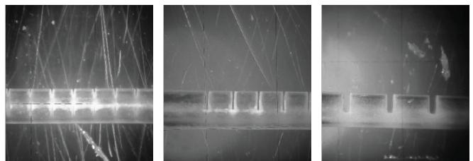
Figure E: Microscope images of the modified catheter tip with 30 µm (left), 50 µm (middle) and 150 µm (right) grooves.
