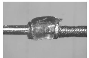
**Fig. 25:** Poly-Pur PS 161 bellow in validation assembly, expanded with 0.5 N
