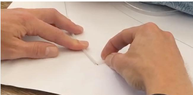
Figure A: 90 degree turn not succeeded due to knot sticking out distally
