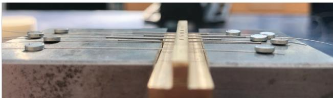
Figure I: Aligning the wires inside the chambers of the mold
