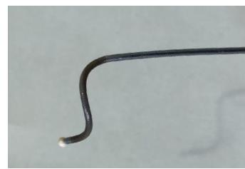
Figure F: new Progreat™ 1, flexible 20cm of the catheter cut off and modified. Resulting curve with 0.5N pulling force (right). Guidewire used is a compatible guidewire of 0.021", with a "permanent bellow" made of 2Component-glue.
