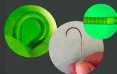
Validation of catheter principle by specialist, with permanent "stopper" in stead of dynamic bellow.
