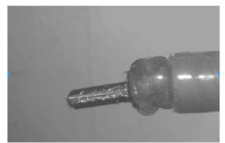
**Fig. 27:** Expanded bellow pulled into the catheter with a force of 0.5N
