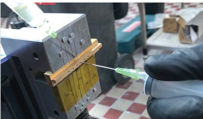
Figure J: Injecting the chambers with rubber while sucking the chamber vacuum
