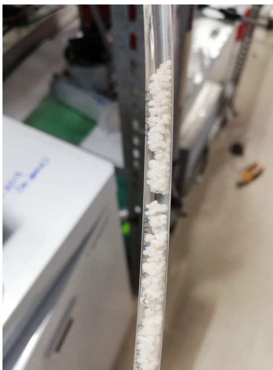
Figure 3.11: Particles in Feed Tube Responsible for Clogging
