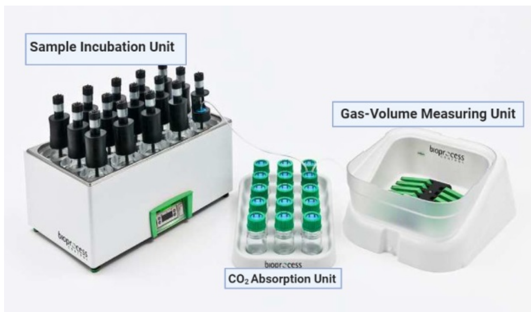
Figure 3.10: Representation of AMPTS-II from Bioprocess Control [5]
