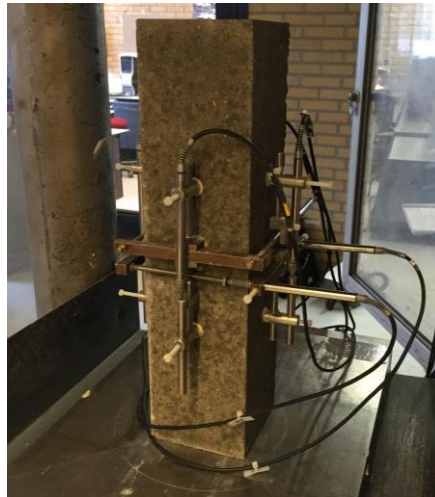
112 113 Figure 1. Testing set-up for elastic modulus measurement on AAC. 114
