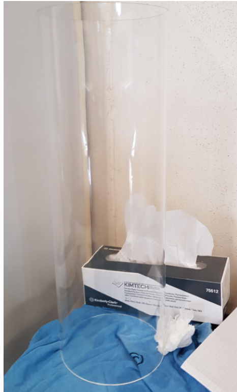
Figure 42: Test tube used in background oriented schlieren test
