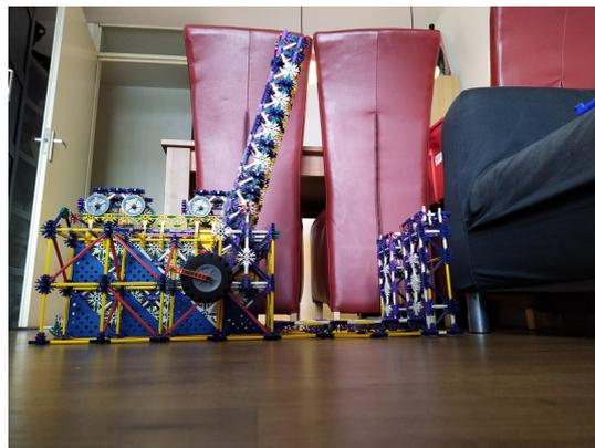
Figure B.1: A k'nex model of the bascule beam rolling gate
