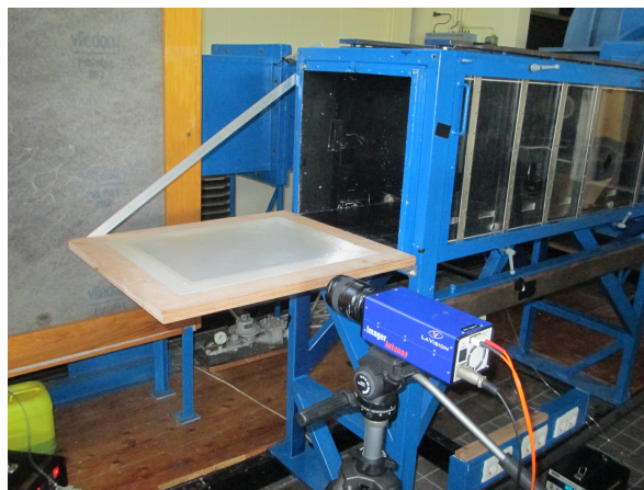
Figure 4.5: Photo of test region, with the glass fiber wall installed
