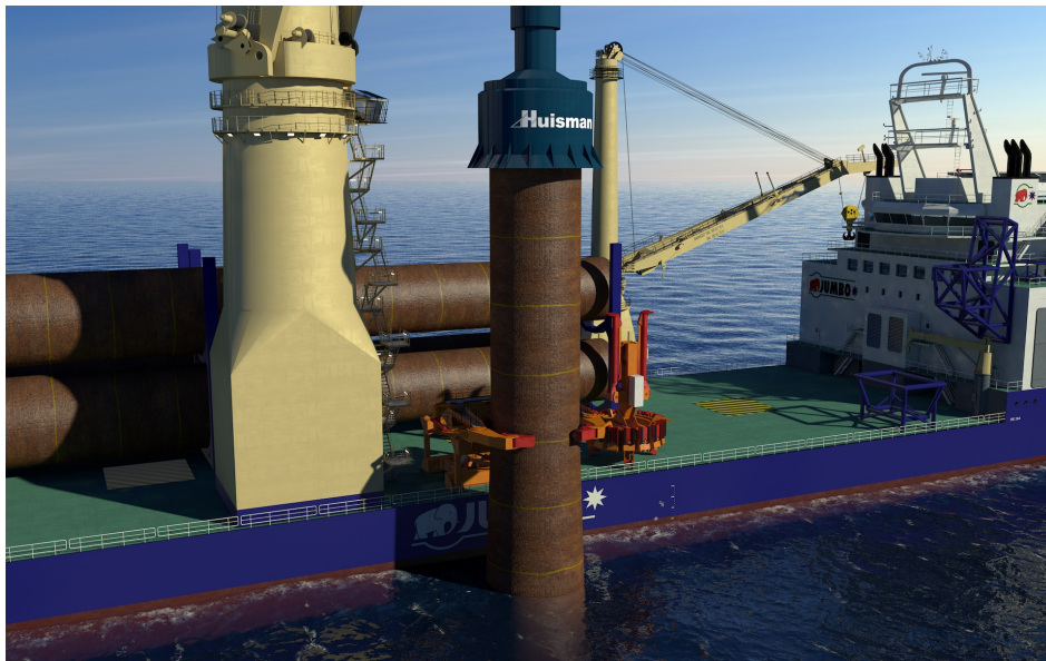
Figure 4-25: Motion-compensated pile gripper of Huisman Equipment B.V.
