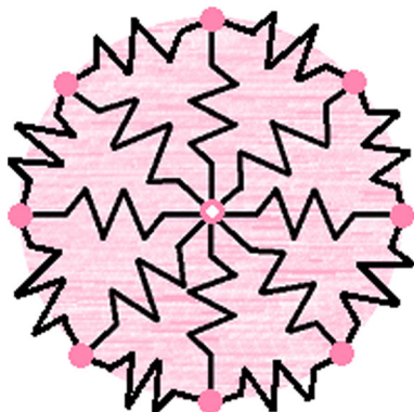
Fig. 1 The division of the cell boundary into mesh points and its connection to the neighbours and to the cell centre as in [48]
