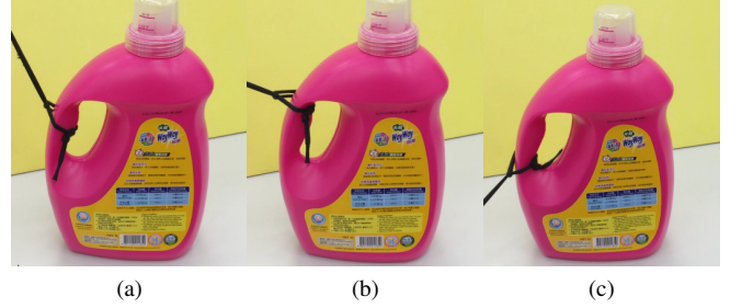
Fig. 11. Caging to grasping process for the detergent container using a rope. The rope starts at a non-stable caging in (a), and then will reach two different stable grasps as shown in (b) and (c), according to whether stretching the rope upwards or downwards.
