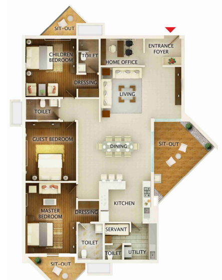
Figure 6.11: The placement of the kitchen near the openings provide effective cooling in the kitchen. Source: archdaily.com
