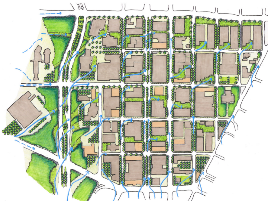
—> Figure 6.2: The open green spaces help in reducing the incoming air temperature and redirecting it through in between paths. Source: DeKay,2012
