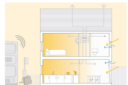
Figure 4.3: Inadequate ventilation because windows are closed. Source: NHBC,2012
