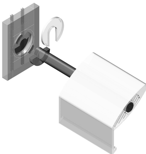
Figure 10.21: Exploded isometric of the self-regulating slat Two types of ventilation slats were considered in order to make automatic modulation during windy and stormy days possible.
