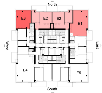
Figure 7.9: Double-sided zones facing North in “layout E” does not have operable windows on the north side, making them more prone to overheating.
