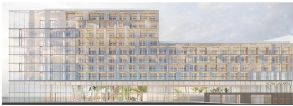
Figure 3: Front view of the modular system. The modules have to maintain its own stability for wind load in both directions.
