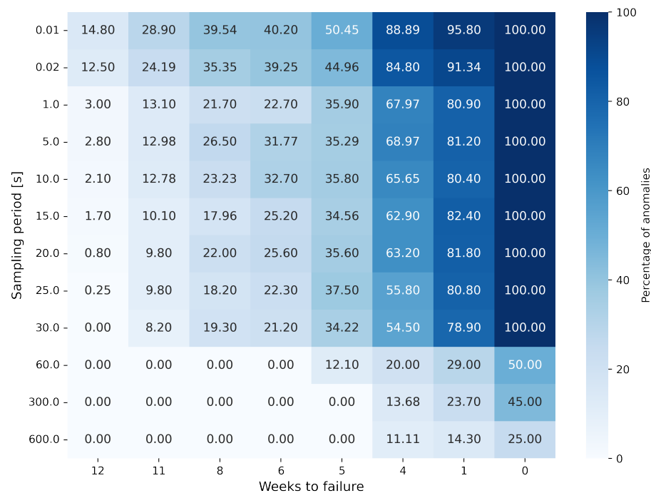
Figure 10: Heat map of the percentage of anomalies detected each week before failure for different SCADA sampling rates
