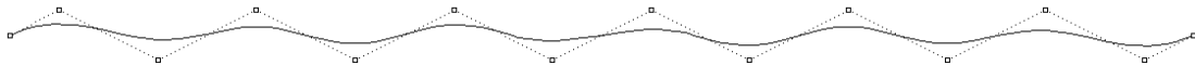
Figure 9.6: Enclosing curve simplification by fitting a NURBS curve through the outer points
