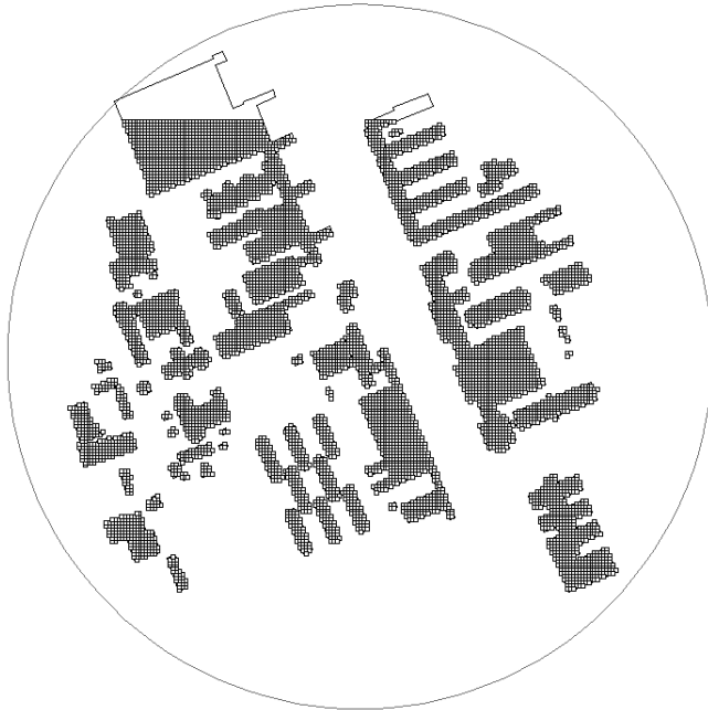
Figure 7.3: Result of the first tool: A 2D model of the research area with the necessary height points lying at the inside of the polygons
