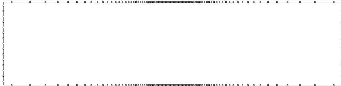
Figure 7.14: Disadvantage of the Rotating Lines method for large models: when a curve is generated through the points, the curve differs from the original model
