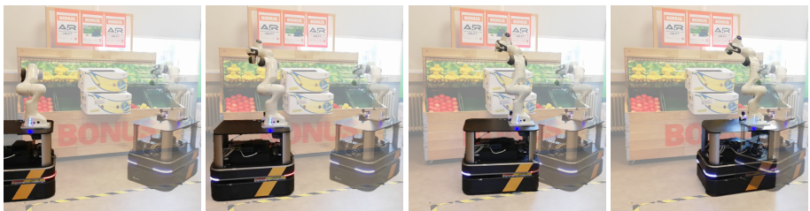
Figure 4.10: Trajectory in mock-up store avoiding obstacles, goal configuration in light grey.
