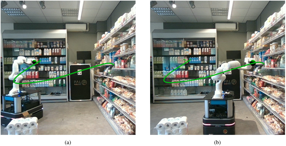
Figure 5.1: Dynamic fabrics for path (green) following with a non-holonomic mobile manipulator. Dynamic fabrics control all actuators simultaneously to follow the end-effector path while keeping a given orientation and avoiding collision with the environment.
