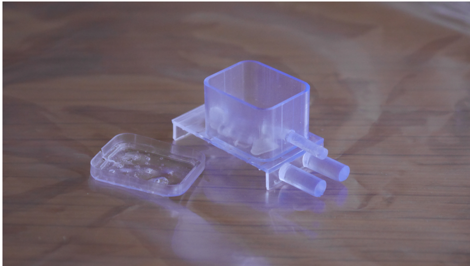
Figure 7.7: The well after 3D printing.
