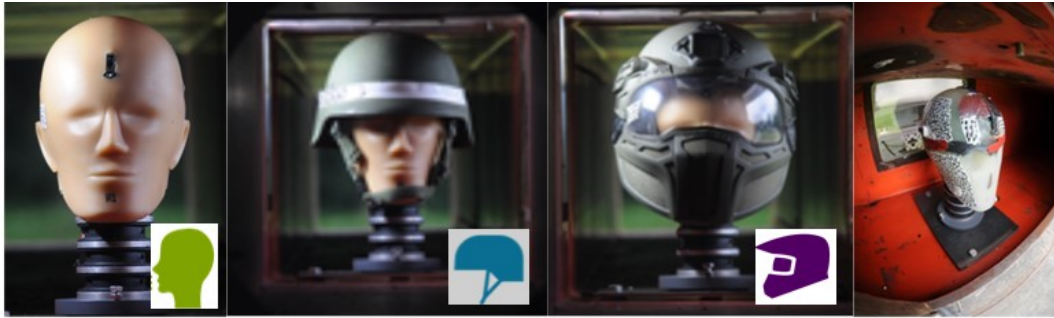
Figure 2.1: Four configurations of the BI2PED during shock tube tests: unprotected, standard combat helmet, full face helmet, unprotected with skin removed[24]
