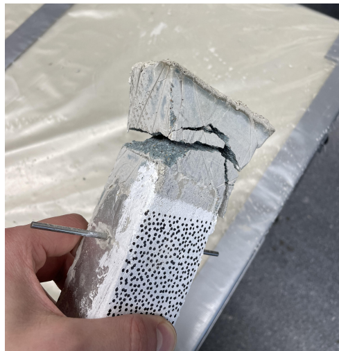
Figure 4.7: The dovetail pulled off the reinforcement during a trial test.
