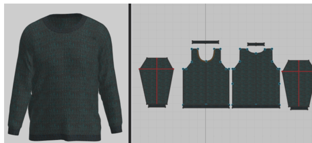
figure 2.14 3D garment (left) created from 2D patterns (right)
