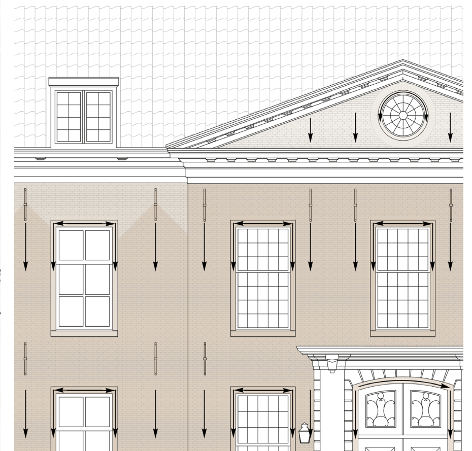
Figure 100: Force distribution in facade view
